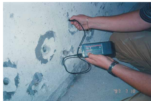
On the left installation of the iron for casting in CLSA – On the right verification tool with the percentage of humidity in the rooms
